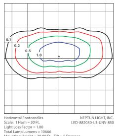
Mounting Height = 30.00 Ft., Tilt = 5 Degrees Maximum Calculated Value = 1.50 Fc Arrangement: Single
