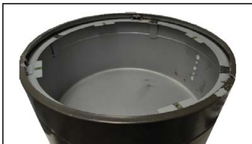
Remove all existing components
