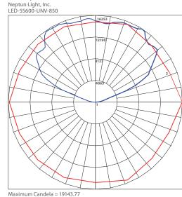
Located At Horizontal Angle = 0, Vertical Angle = 147.5 #1 - Vertical Plane Through Horizontal Angles (0-180) (Through Max. Cd.)
