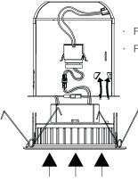
For existing 6" in. diameter cans / downlights For screw-in Medium (E26) base socket
