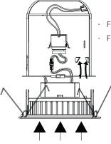
For existing 5 & 6" in. diameter cans / downlights For screw-in Medium (E26) base socket
