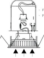
For existing 4" in. diameter cans / downlights For screw-in Medium (E26) base socket
