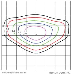
Scale: 1 Hash = 30 Ft. Light Loss Factor = 1.00 Total Lamp Lumens = 18002.32 Mounting Height = 30.00 Ft., Tilt = 5 Degrees Maximum Calculated Value = 5.08 Fc
