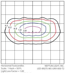
Mounting Height = 40.00 Ft., Tilt = 5 Degrees Maximum Calculated Value = 2.52 Fc Arrangement: Single
