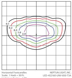
Light Loss Factor = 1.00 Total Lamp Lumens = 14281.5 Mounting Height = 30.00 Ft., Tilt = 5 Degrees Maximum Calculated Value = 4.08 Fc
