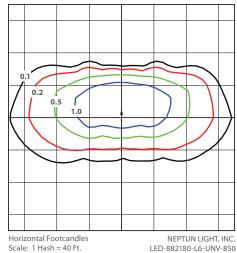
Light Loss Factor = 1.00 Total Lamp Lumens = 18351.2 Mounting Height = 40.00 Ft., Tilt = 5 Degrees Maximum Calculated Value = 1.76 Fc Arrangement: Single
